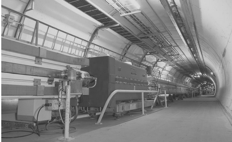
13. A view inside the 27-km (17-mile) circular tunnel of CERN's Large Electron Positron (LEP) collider, which ran from 1989 to 2000. The electrons and positrons travelled in opposite directions in the beam pipe through hundreds of brown and white bending magnets (dipoles) and blue focusing magnets (quadrupoles). Originally LEP accelerated the beams to a total collision energy of around 90 GeV, but by the time of its final shutdown in October 2000 it reached more than 200 GeV.
